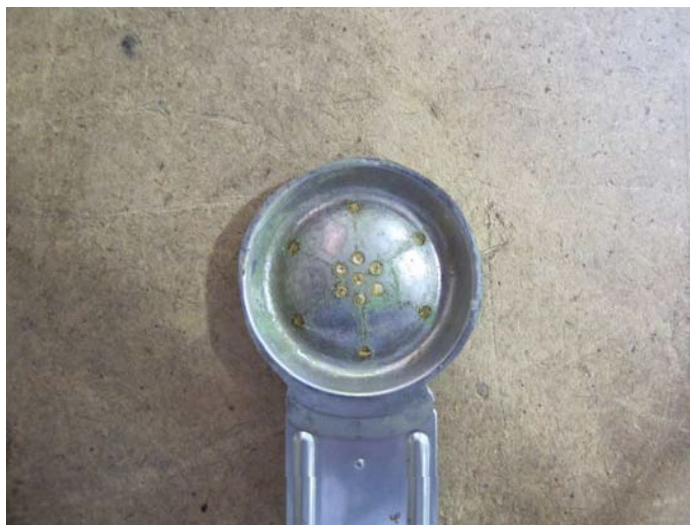
Figure 46—Disk Subjected to Corrosion
