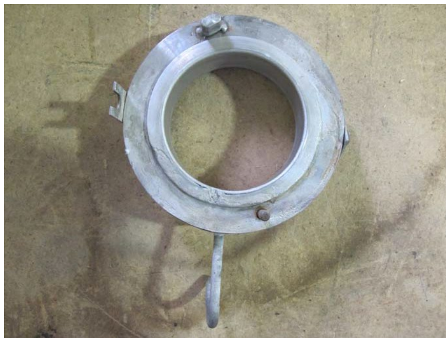
Figure 48—Rupture Disk Holder Subjected to Corrosion
