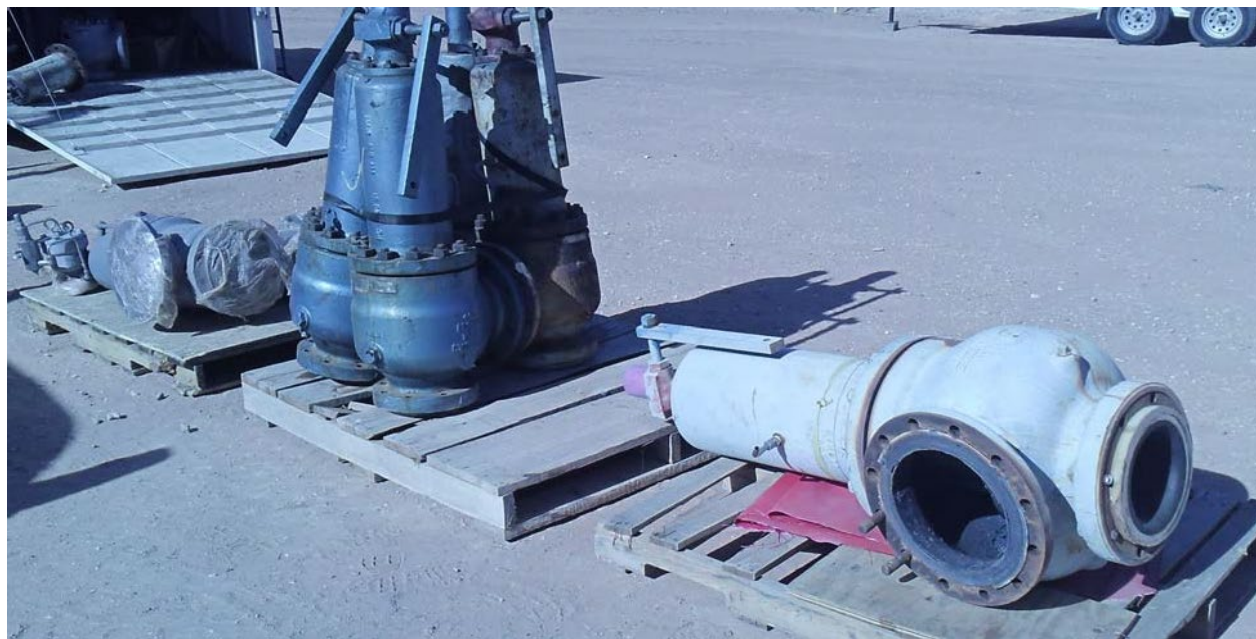
Figure 36—Improper Storage of Valves
