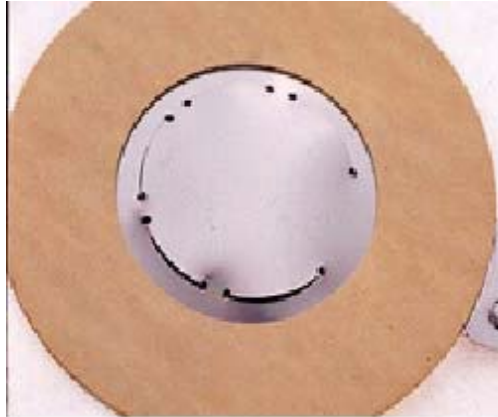
Figure 45—Operating Ratio Exceeded—Tabs Are Stretched
