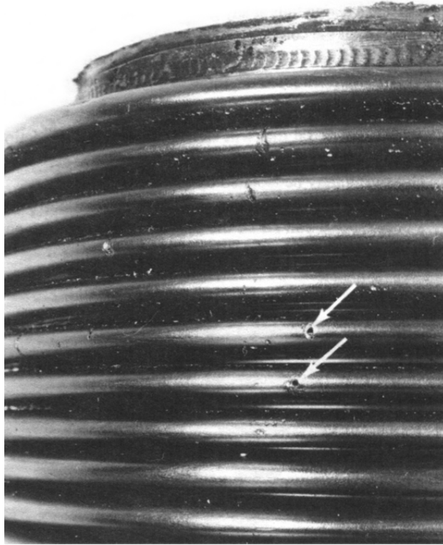
Figure 25—Pit-type Corrosion on 18Cr-8Ni Steel Bellows
