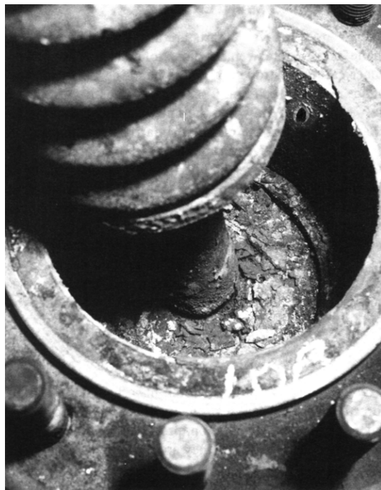
Figure 34—Moving Parts of Valve Fouled with Iron Sulfide ( \text{FeS}_2 )
