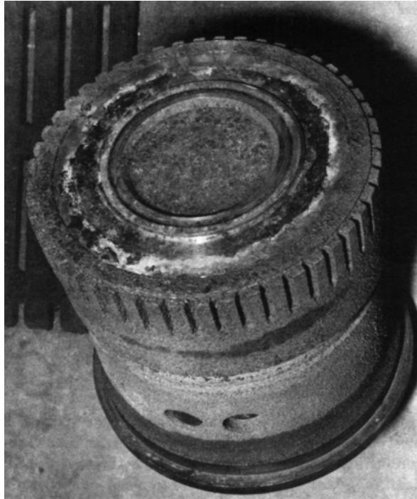
Figure 35—Disc Frozen in Guide Because of Buildup of Products of Corrosion in Sour Oil Vapor Service
