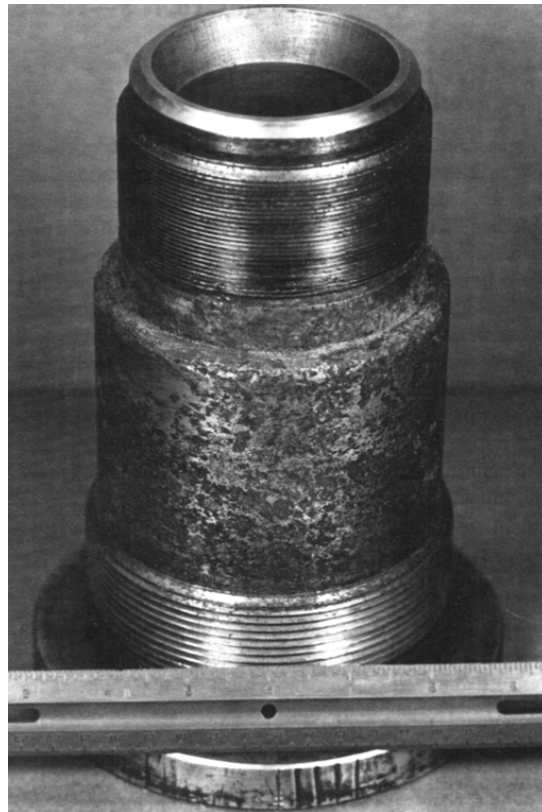
Figure 22—Chloride Corrosion on 18Cr-8Ni Steel Nozzle (with Machined Seating Surface)
