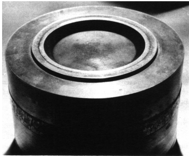
Figure 28—Seating Surface of Disc Deformed by Chattering
