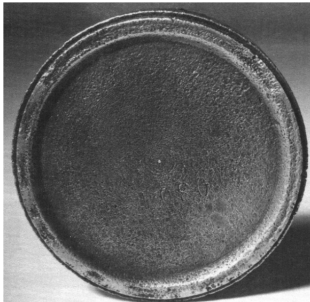
Figure 24—Chloride Attack on 18Cr-8Ni Steel Disc
