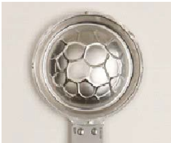
Figure 44—Operating Ratio Exceeded, Then Subjected to Vacuum
