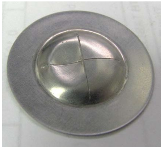
Figure 50—Dent Caused by Water Freezing in Discharge Line
